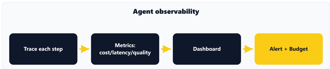
Figure 20 — Trace every LLM/tool call, emit the three pillars of metrics, and alert on budgets.
