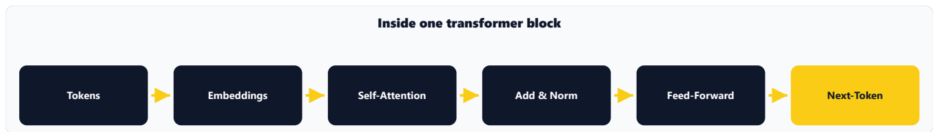
Figure 2 — Data flow through a transformer block. Self-attention lets every token weigh every other token before the feed-forward layer refines the representation.
